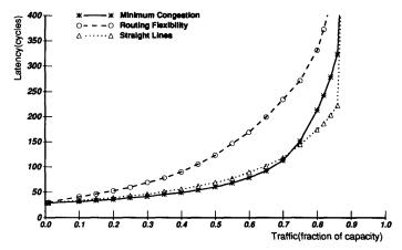
Fig. 8. Latency as a function of offered traffic for three selection functions. Simulations were performed using dynamic adaptive routing and random traffic.
