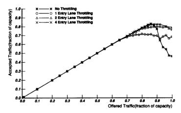
Fig. 6. Throughput as a function of offered traffic for a 16-ary 2-cube network using dynamic adaptive routing with varying degrees of throttling. Throttling reduces peak throughput by restricting the entry of new packets into the network.
