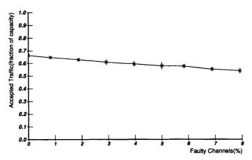
Fig. 10. Throughput versus percent faulty channels for a 16-ary 2-cube network with random traffic and throttling with a single entry lane. Each point gives the mean throughput of 20 randomly generated faulty networks. The error bars show the  $1\sigma$  points of each distribution.
