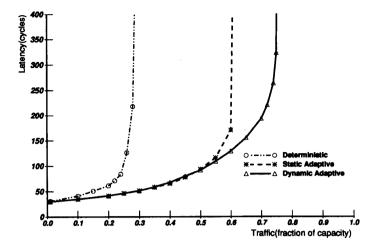
Fig. 5. Latency versus accepted traffic for a 16-ary 2-cube under bit reversal traffic. Deterministic dimension order routing is compared with static and dynamic adaptive routing. This nonuniform traffic pattern causes deterministic routing to perform very poorly, saturating at about 25% capacity. Static and dynamic adaptive routing achieve three times this performance (saturating at 60% and 75% capacity, respectively) by routing to distribute the network load.
