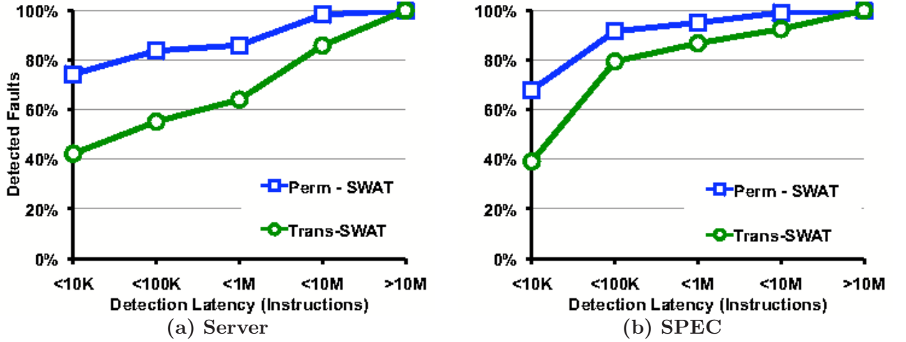
Figure 3.4: Detection latency for detected non-FPU permanent and transient faults in (a) Server and (b) SPEC workloads. Over 98% of the detected faults are detected at a latency of < 10M instructions, making them recoverable with hardware checkpointing.
