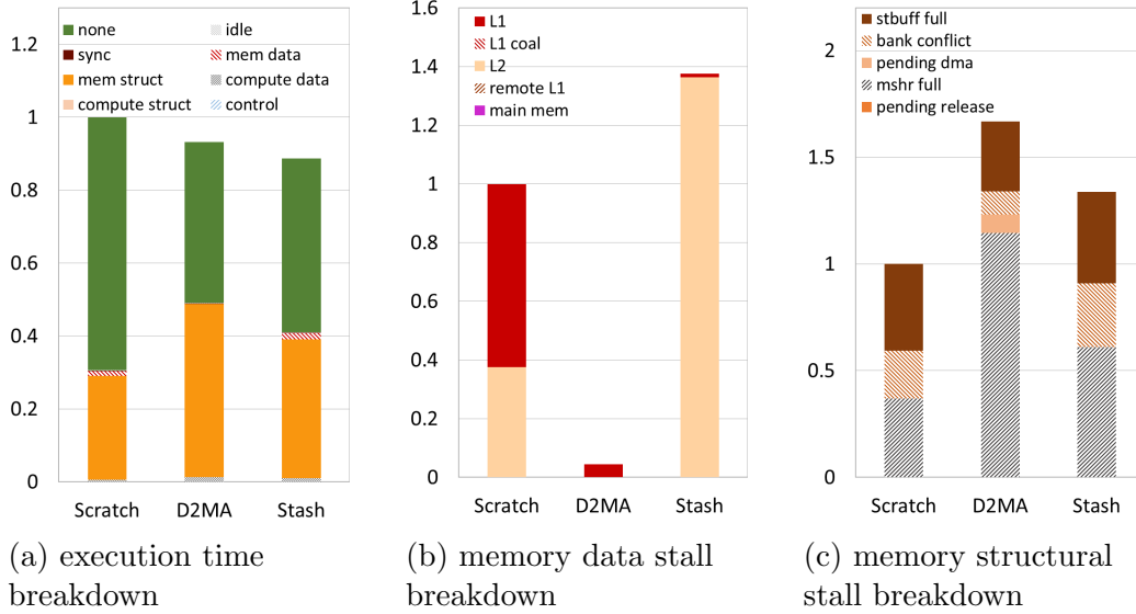
Figure 6.3: Stall cycle breakdowns for implicit microbenchmark (normalized to baseline scratchpad).
